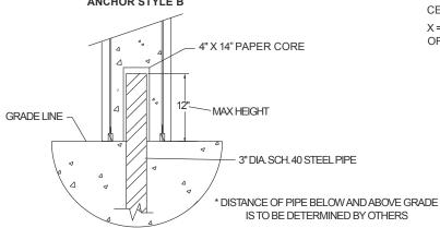
NOTE: THIS TYPE ANCHORING IS ALSO USED AS A BARRICADE. BOLLARD HELD IN PLACE BY STEEL PIPE STEEL PIPE MUST BE ANCHORED IN CONCRETE FOOTING
