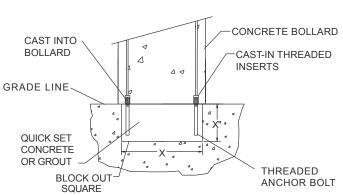
NOTE: THIS TYPE ANCHORING IS NOT USED AS BARRICADE.
