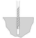
Drill 3/8" diameter holes 3" deep into surface. Make sure the holes are at least 3" away from any cracks in the base material.
