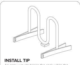
An easy way to brace the rack while the grout sets is to bolt two 1x4" boards together at one end and clamp them onto the rack like a clothes pin.
