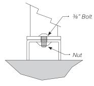
Put bolts through Hoop Rack flange holes and beams so bolt head faces up. HAND tighten the nuts using new flange nuts.
