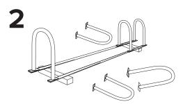
Place Hoop Racks on beams so holes in rack flanges line up with beam slots
