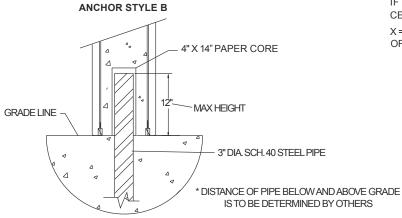
NOTE: THIS TYPE ANCHORING IS ALSO USED AS A BARRICADE. BOLLARD HELD IN PLACE BY STEEL PIPE STEEL PIPE MUST BE ANCHORED IN CONCRETE FOOTING TYP. 12" DIA. CONCRETE BOLLARD SAME
