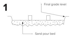
Place corrosion resistant sleeve (min. 4" inside diameter) in sand pour bed in exact location where rack will be installed. Make sure top of sleeve is at same level as desired finished concrete surface. Fill sleeve with sand to keep it in place and prevent it from filling with concrete.
